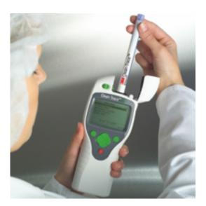
The 3M<sup>™</sup> Clean-Trace<sup>™</sup> ATP system provides an objective and highly reliable indication of cleanliness on work surfaces (and thus microbial risk) within seconds of sample collection.
