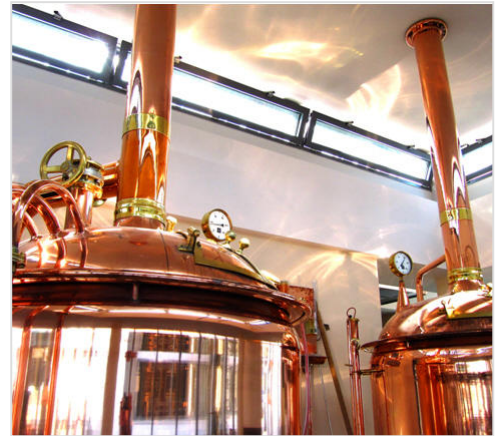
Brew kettles made of copper. At this stage hops are added to the wort before being boiled. Once the liquid has achieved the correct aroma, it is transferred to the heat exchanger to be cooled down.
