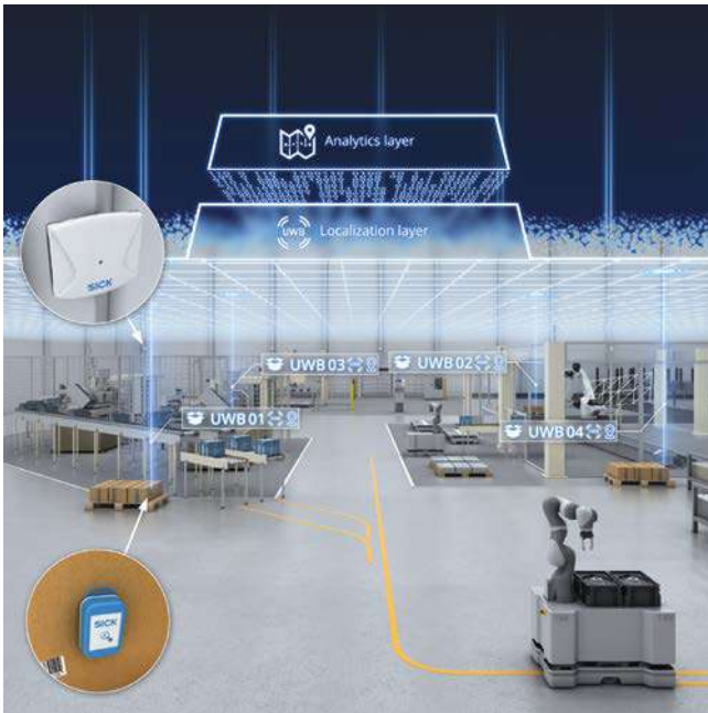
Fig. 8: Determining the absolute location of assets using UWB tags and UWB receiver antennas (LOCU1xx and LOCU2xx from SICK). The data collected can subsequently be visualized, analyzed, and further used in the Asset Analytics platform from SICK.
