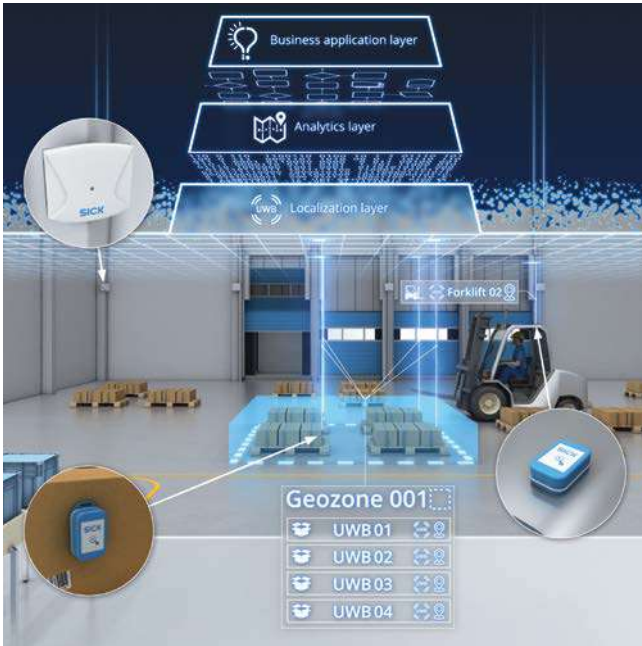
Fig. 10: The data collected in various geozones are forwarded by the Asset Analytics localization software to higher-level ERP systems and MES.
