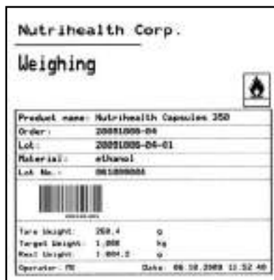
A newly printed weighing label helps guarantee component identification
