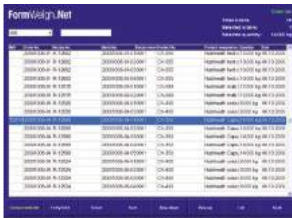
After successful log-in, planned production orders are presented to the operator
