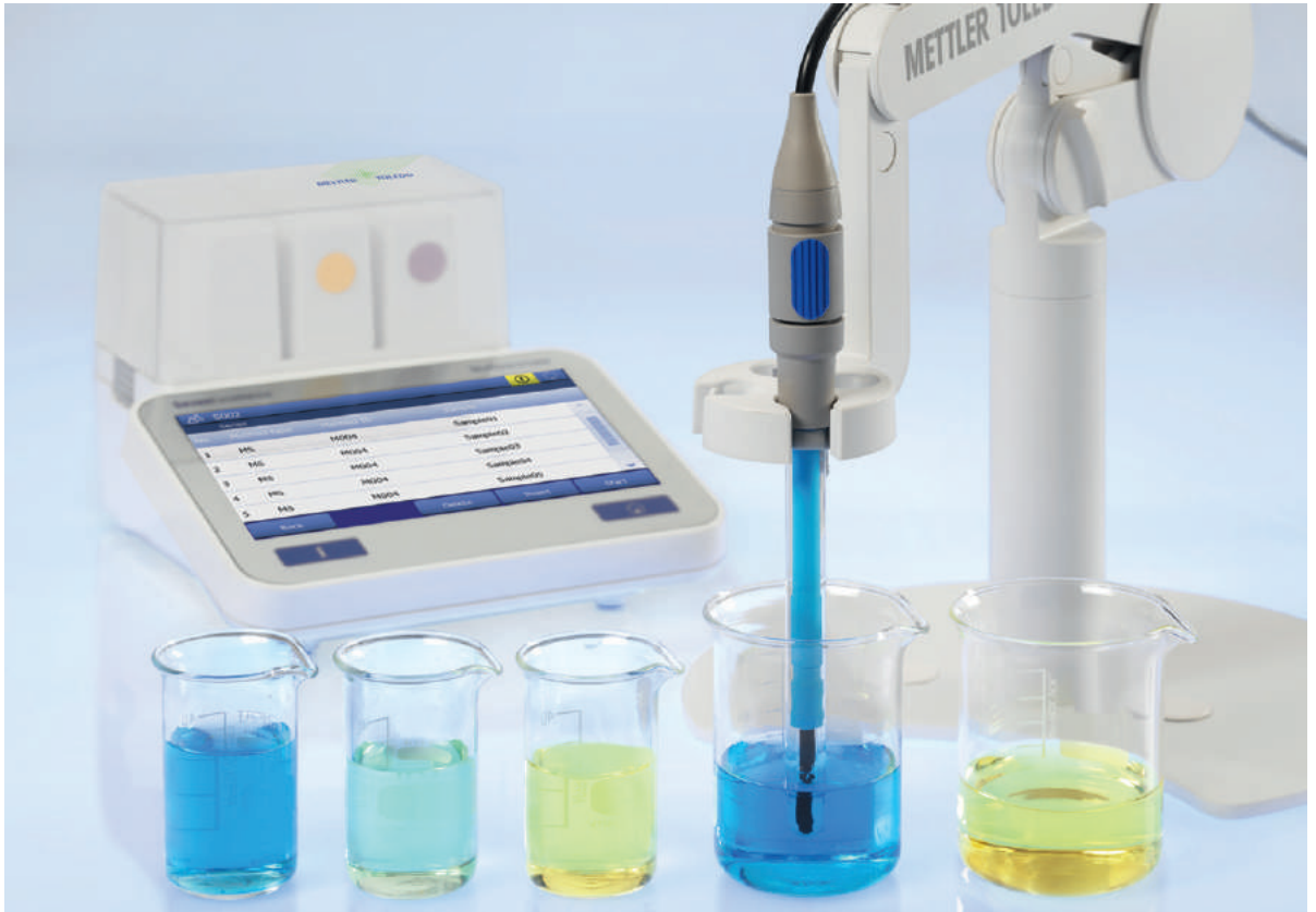
Figure 17: SevenExcellence meter and InLab® electrode during calibration.
