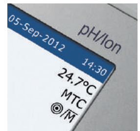
Figure 8: Temperature and MTC indication on a pH meter.
