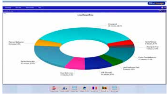
The above iDSnet Manager dashboard provides information on causes of unplanned downtime assigned by the operators via reason codes.
